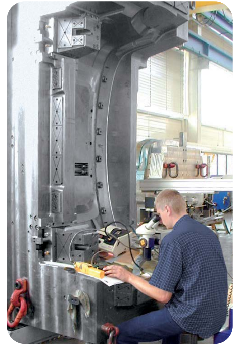
Processing of a 20t injection mold for bumper production.
